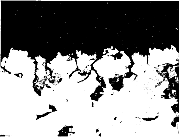
FIG. 10. Stress corrosion cracks (partly transgranular) in mild steel. 4N \text{Ca}(\text{NO}_3)_2 , pH 3.7 (at 25°C), 102°C, e_{\text{H}} - 0.10V. ( \times 400 )
