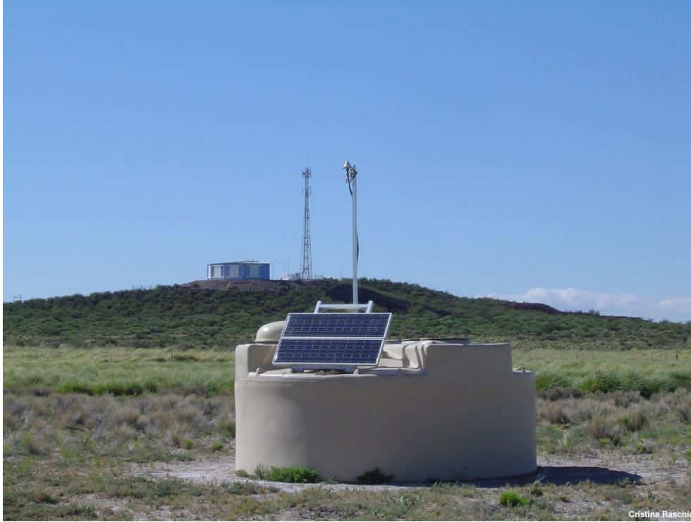
Figure 1.5: Water-Cherenkov detector at the Pierre Auger Observatory and its main components. Picture adapted from [41].
