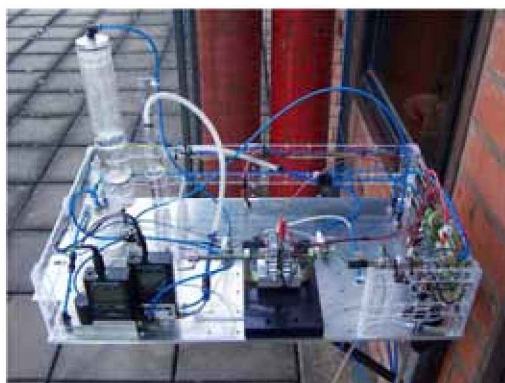
FIG. 3. View of the fuel monocell test station showing the humidifiers, flow controls and associated circuits.
