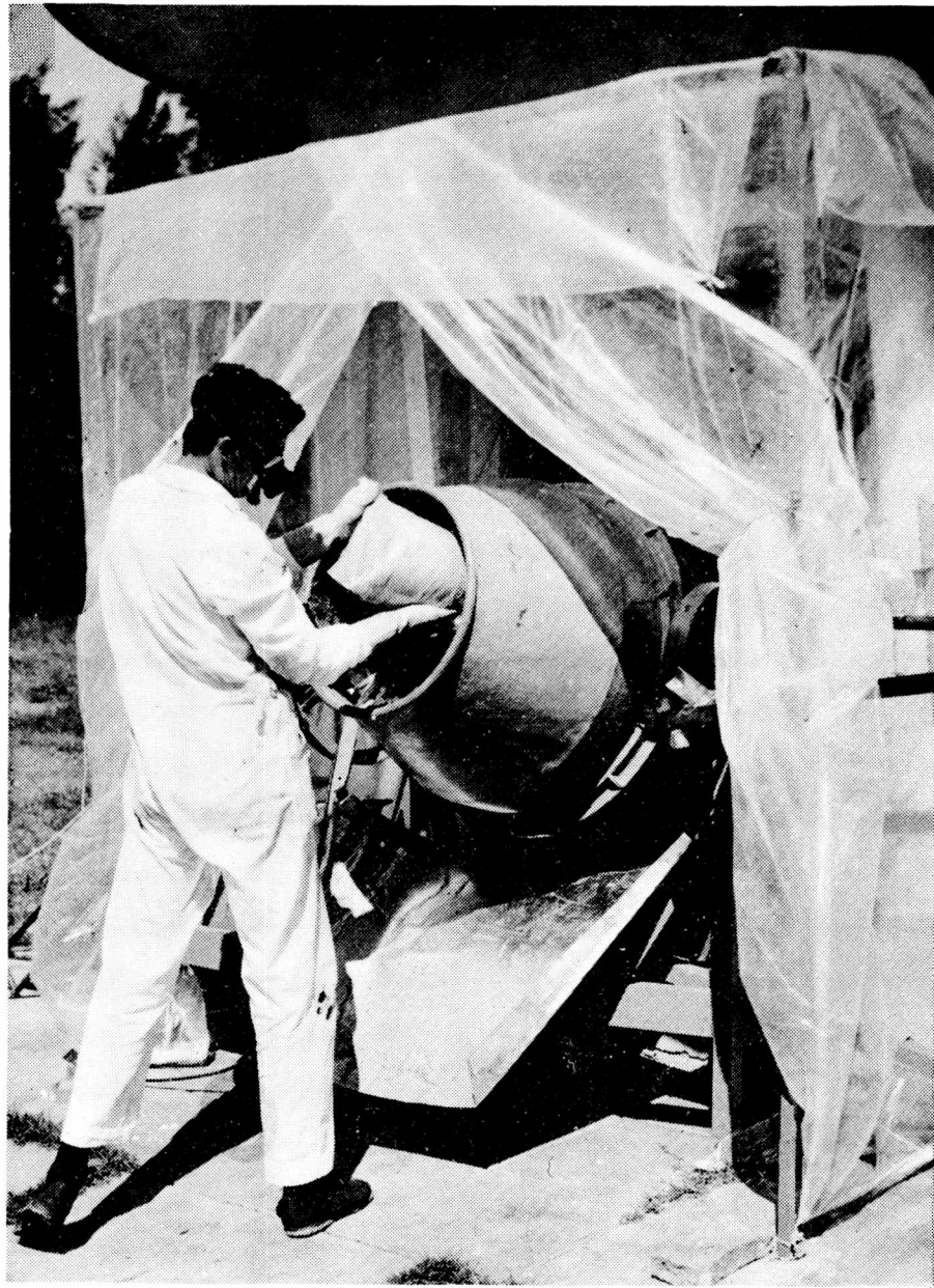
FIG. 4-9 INACTIVE SEDIMENT IS PLACED IN THE MIXER FOR LABELLING WITH Ag-110.
