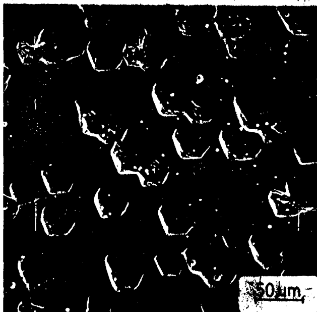
FIGURE 3 — Localized corrosion of high purity zinc in deaerated 0.1\text{M} NaCl solution ( \text{pH} = 9.0 ). Specimen exposed 18 hours at -0.91 V plus 40 minutes at -0.67 V.
