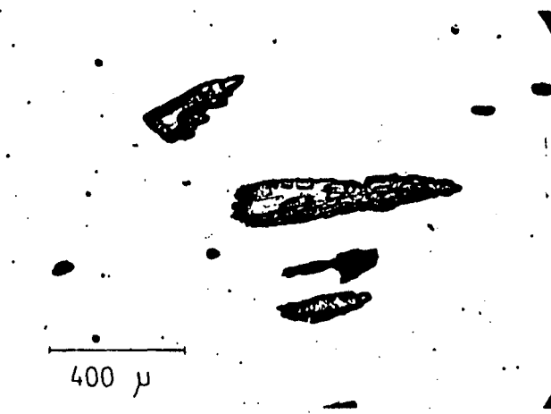
FIGURE 9 - Pitting of pure Al in a 0.9M \text{NaNO}_3 plus 0.1M NaCl solution. The pitting potential is the same as for pure \text{NaNO}_3 solutions, but the pits are arrow-shaped and their interior is covered with a thick layer of corrosion products.
