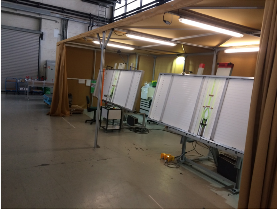
Figure 4.7: Construction area for the assembly of the 661 SSDs at the Institute for Astroparticle Physics at the KIT. The two assembly tables can be tilted up to \sim 80^\circ to avoid a bending of the fibers during the gluing process. The surrounding curtains provide a protection of the sensitive scintillator bars and fibers against UV radiation. Taken from Ref. [125].
