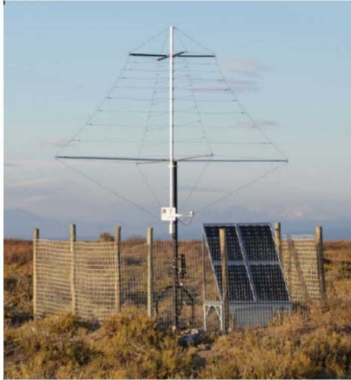
Figure 3.9: Photo of an LPDA installed in the AERA. Taken from Ref. [86].
