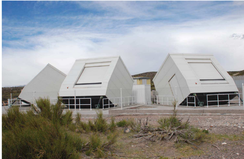
Figure 3.3: The three telescopes of the HEAT enhancement in upwards position and closed telescope shutters. Taken from Ref. [72]
