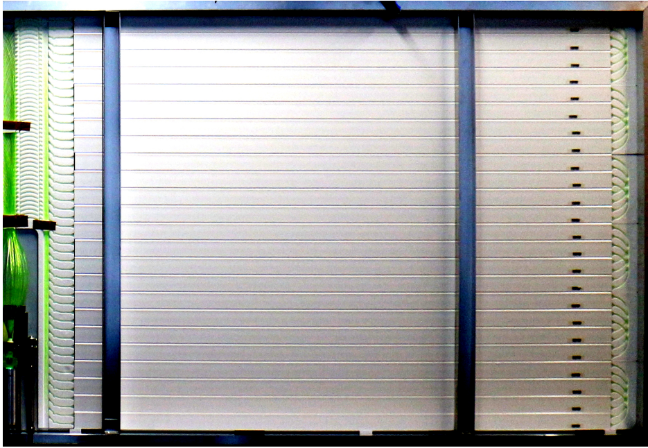
Figure 3.12: Top view of a completed wing of an SSD, including the 24 narrowly arranged scintillator bars, the WLS fibers inserted in the bars and routed by the XPS forms towards the readout device. Taken from Ref. [108].
