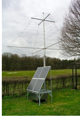
Figure 3.29: A radio station prototype. The log-periodic dipole antenna and solar panels are visible. The electronics and digitizer are placed in the aluminum box beneath it [225].
