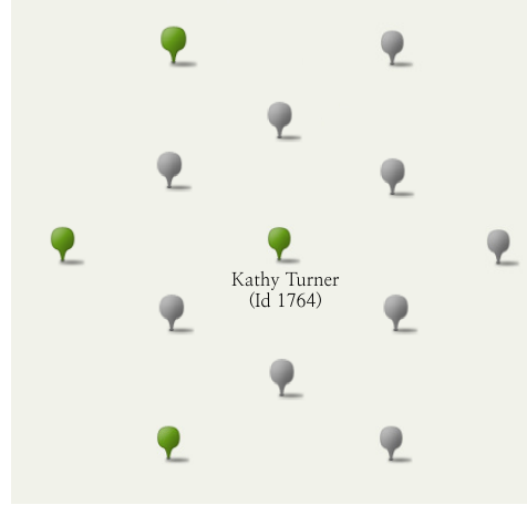
Figure 3.17: The schematic map of the SD-433 array. The green (gray) icons represent the location of WCDs with (without) an associated MD station. The Id 1764 WCD and its associated MD station are located in the center of the SD-433 hexagon.
