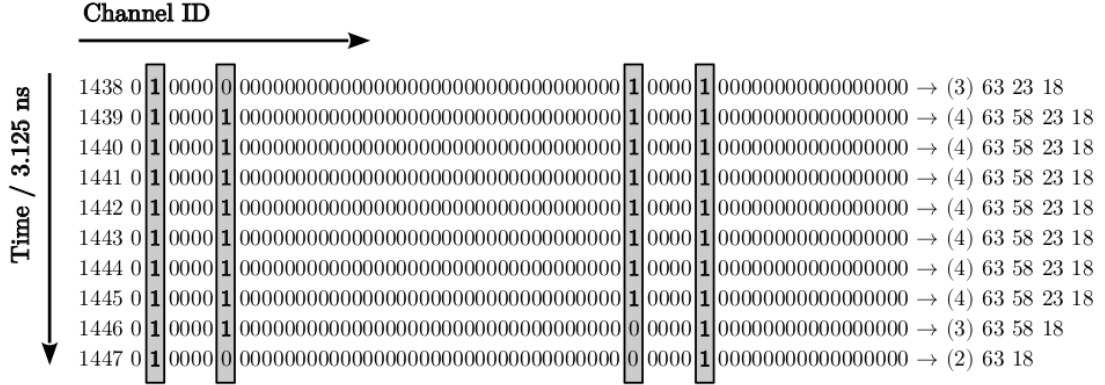
Figure 3.9: Example of a binary-mode output signal from a UMD station. Each column corresponds to one of the 64 channels, and each row represents a time bin. Figure adapted from [43].
