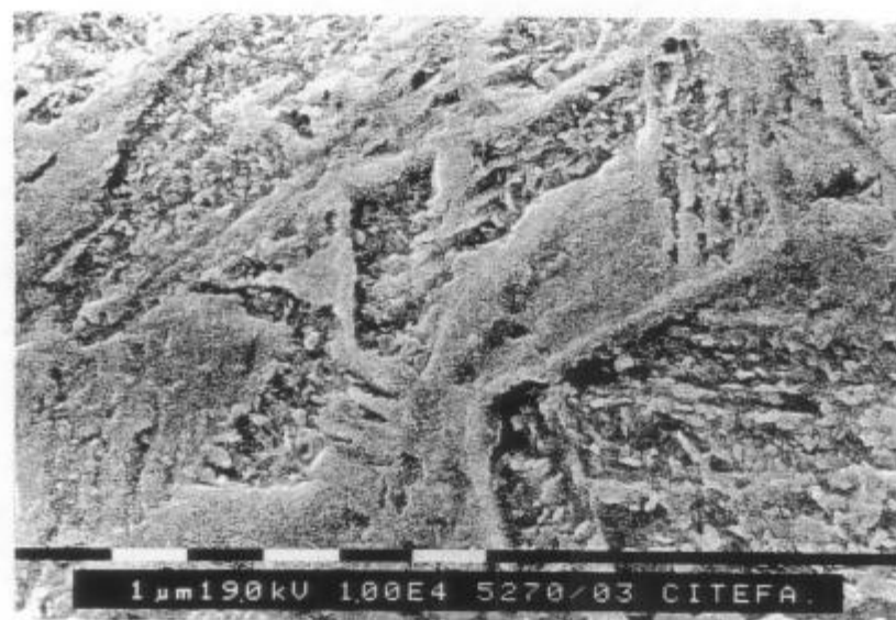
Figura 3.17c: Acero A24, Venf. = 2.5 °C/s. (10000X).
