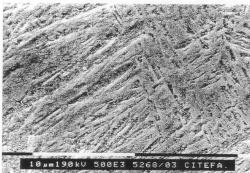
Figura 3.17b: Acero A24, Venf. = 2.5 °C/s. (5000X).
