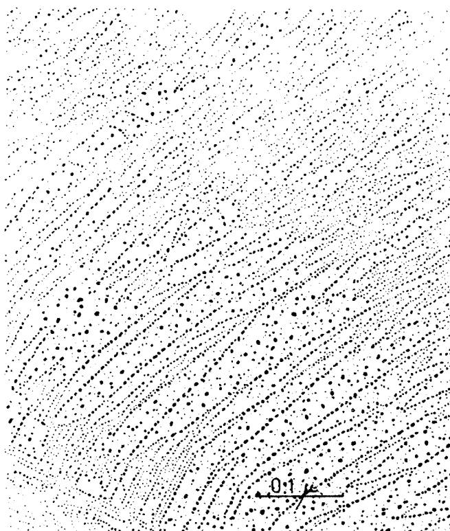
Restarting zone with inclined steps. Standard decorated replica of a NaCl crystal.
