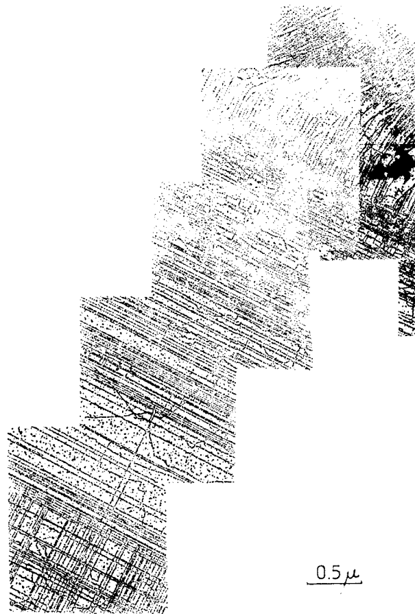
Composite electron micrograph of a decorated replica of a NaCl crystal showing tartan-pattern, stop-band and restarting zones.
