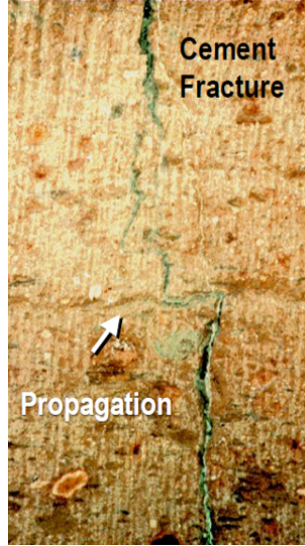
Figure 4.6: Fracture growth across discontinuities forming an offset, obtained during hydraulic fracture experimental tests, performed by Warpinski (2011) .
