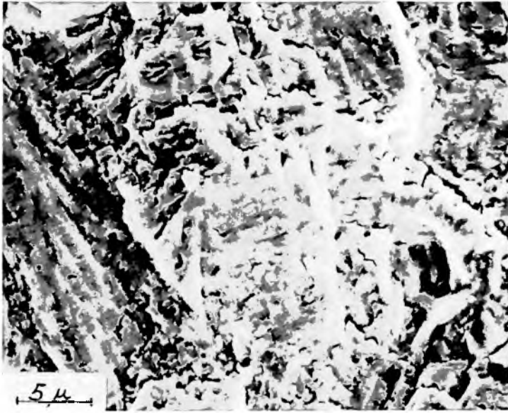
Fig. 8. DIN 1.4550: fracture surface of a low-cycle mechanical fatigue crack.
