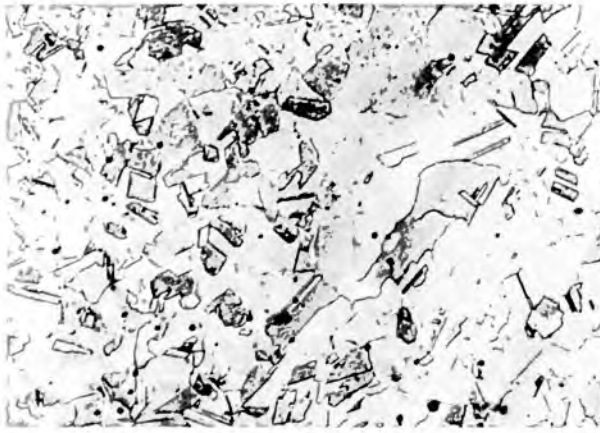
Fig. 5. DIN 1.4550: austenitic stainless steel microstructure with partial recrystallization ( \times 100 ).
