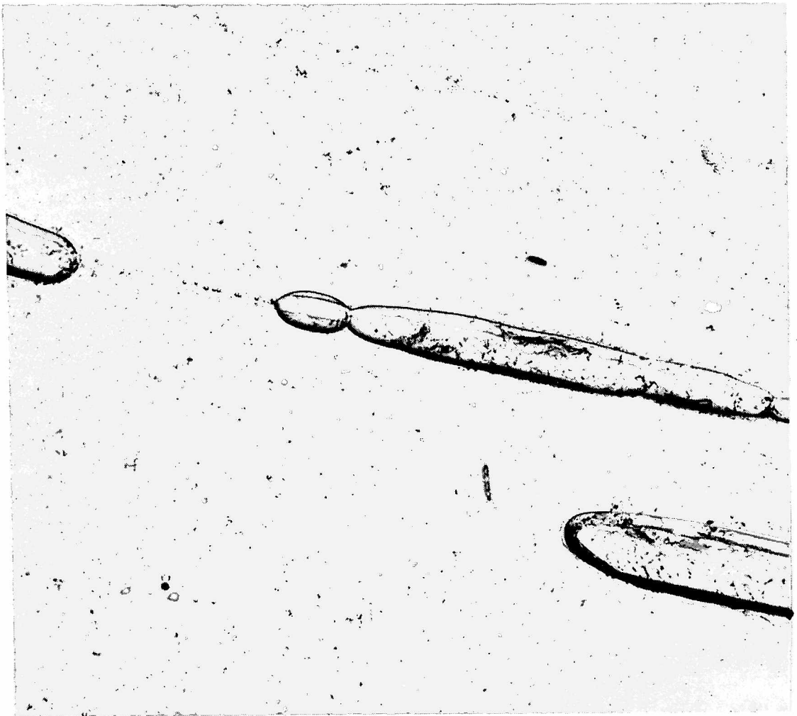
FIGURE 14.- Aluminum strained in 1 M \text{NaNO}_3 solution above the pitting potential ( E = 1.8 \text{ V n.h.e.} ). Pitting nucleates on the slip steps. Oxide replica, 4000 X (162).
