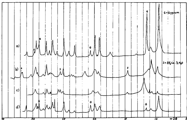
FIG. 4. X-ray diffraction goniometer traces of impure ranquillite.
