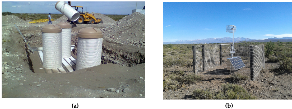
Figure 1.9: (a) Photograph of AMIGA detectors during their installation in the field. Modules of plastic scintillators are buried at around 2.3 m. The tubes are used for accessing the electronics. Taken from [34]. (b) Picture of an antenna of the AERA radio detector.
