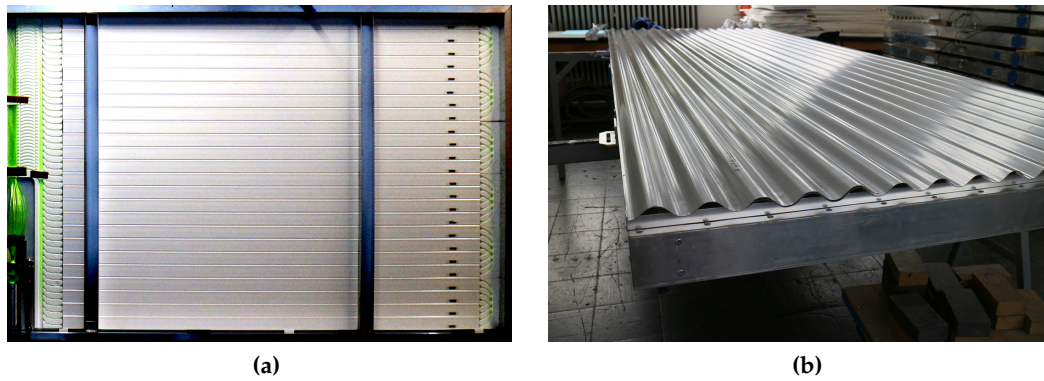
Figure 2.7: (a) Top-down view of the right module of a SSD. The 24 scintillator bars lay together and are interconnected with the WLS fibers. The “U” routine may be observed on the right side of the picture. Fibers are then routed back to the PMT which is placed at the bottom left corner in the picture. Photo courtesy of David Schmidt. (b) Roof and aluminum housing of the SSD (see text for details). Picture taken from [74].
