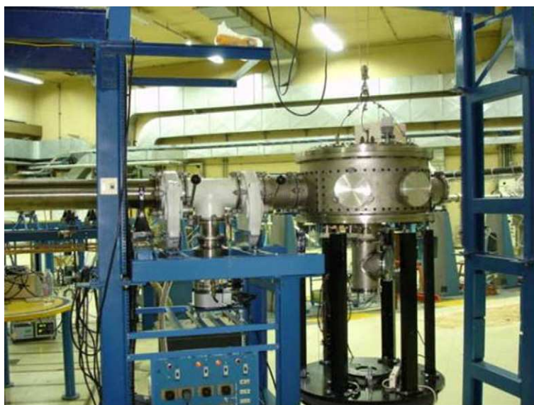
Fig. 4. 76-cm vacuum chamber installed on one of the Tandar accelerator beam lines.
