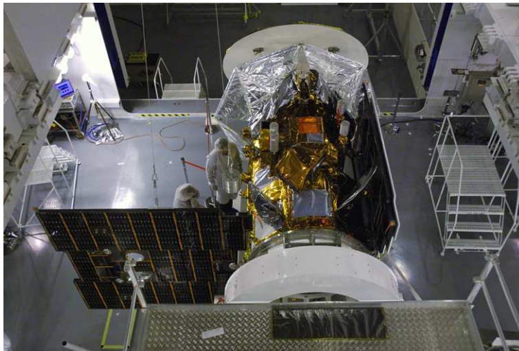
Fig. 20. Solar panels mounted on SAC-D satellite, at the launch site at Vandenberg, California, USA. 2
