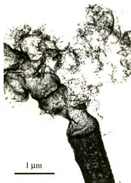
Fig. 2. Bright field TEM image for an LSMO hollow NAN. Attached to its end, the tip shows a structure resembling bubbles, suggesting the escaping of gases during the evaporation of the precursor while the thermal treatment is taking place.
