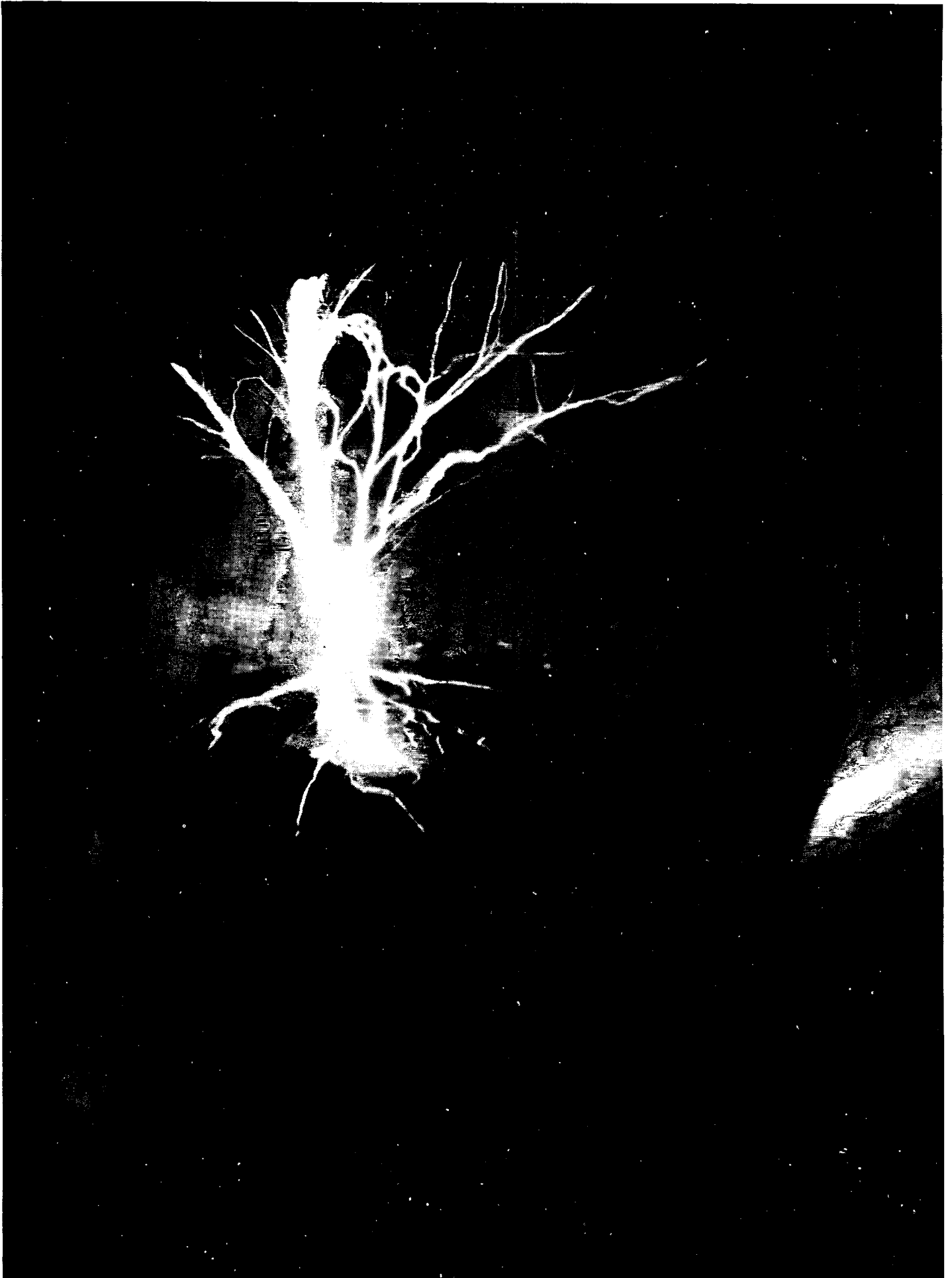
Fig. 6. A terminal spark during column voltage tests.
