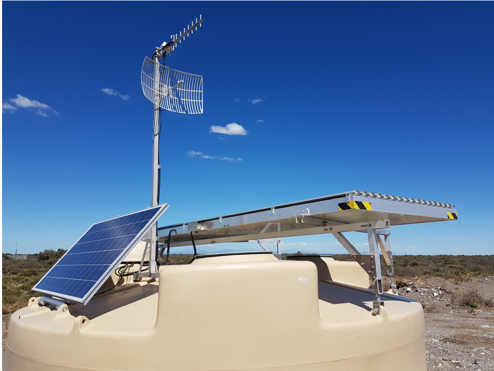
Figure 2.7: A sample photograph of an SSD deployed in the standard array above a WCD.
