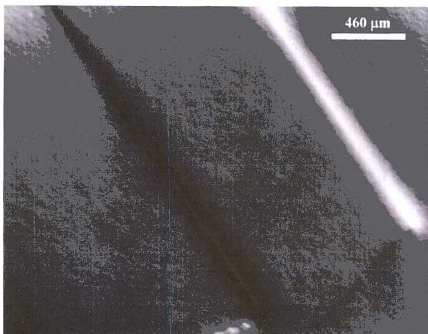
Figura 6.66. \text{Cd}_{0,96}\text{Zn}_{0,04}\text{Te} , v = 3,32 \text{ mm/h} (oblea 2, macla)
