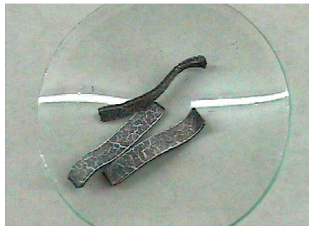
Fig 3. First calcined miniplate to 750^\circ\text{C} (5h).
