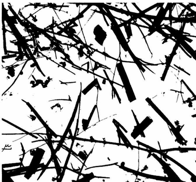
FIG. 1. Electron micrograph obtained with sanjuanite crystals.
