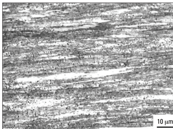
(g) A longitudinal metallographic section of the steel strand.
