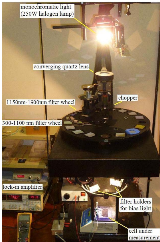
Figure 1: General view of the measurement equipment. The monochromatic light is aligned with all pieces: the converging lens, the chopper disc, the first and second filter wheels and, finally, the sample on the thermostated base plate.
