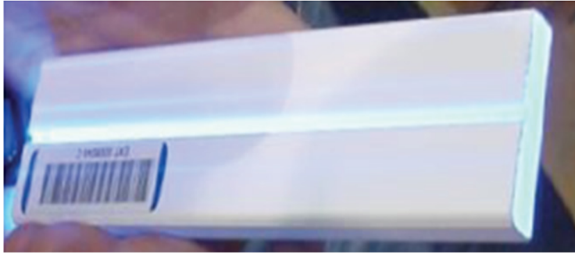
Figure 3.7: Piece of scintillator strip used in the UMD modules.
