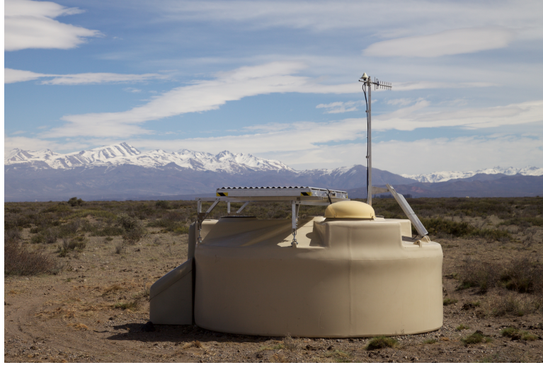
Figure 3.11: Surface Scintillator Detector station of AugerPrime All Surface Detector stations will be equipped with a plastic scintillator bar on top to enhance separate measurements of the electromagnetic and muonic shower component.
