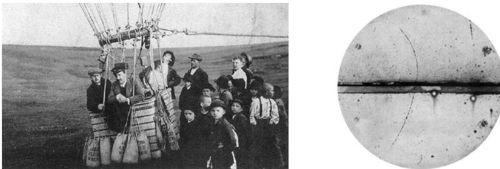
Figure 1.1: Left: Victor Hess, at the center, departing from Vienna about 1911, soon discovering the penetrating ionizing radiation from outer space. Right: Anderson’s cloud chamber picture of cosmic radiation from 1932 showing for the first time the existence of the positron (picture taken from [4]). The particle enters from the bottom, strikes the lead plate in the middle and loses energy as can be seen from the greater curvature of the upper part of the track. The curvature was induced intentionally by a magnetic field.
